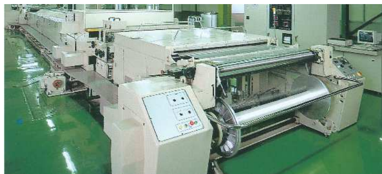
Sizing process (warping sizer)
