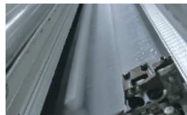
Weaving process (waterjet loom) The sized thread is woven into textiles.
